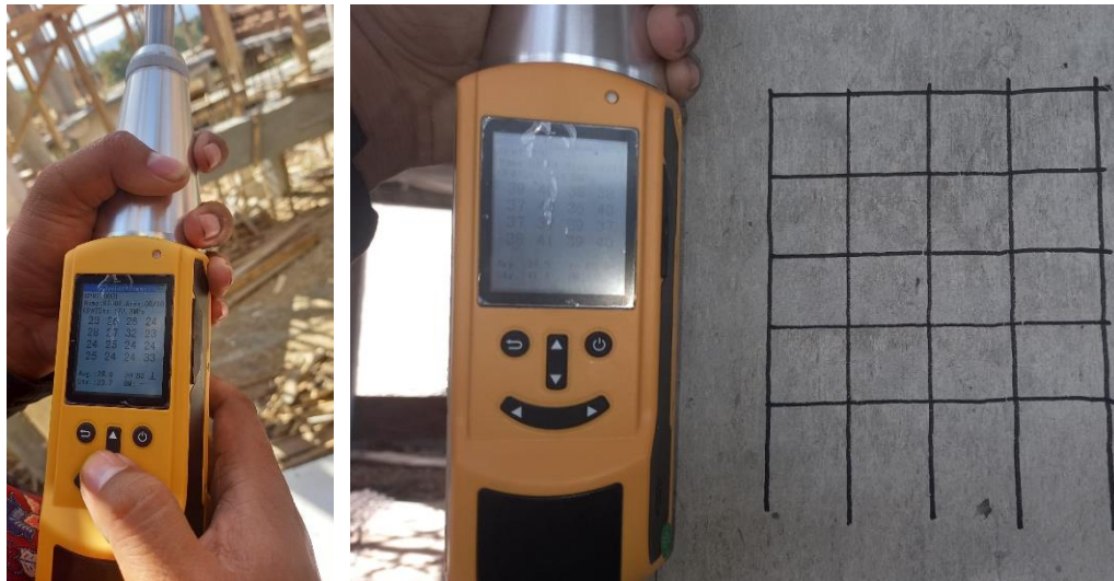
Gambar 5. Data Uji Hammer Test 2
