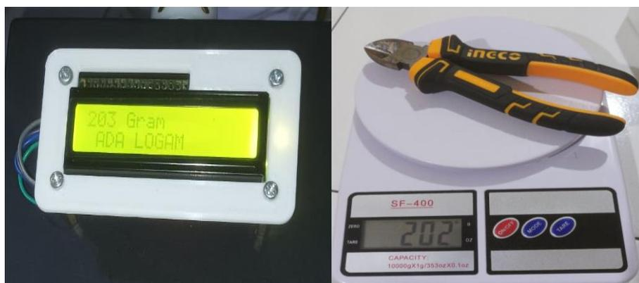
**Gambar 13. Hasil Pengujian Timbangan Benda 2 (Tang Potong)**
