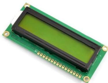
**Gambar 5. LCD (2x16)**
