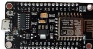
**Gambar 7. NodeMCU ESP8266**
