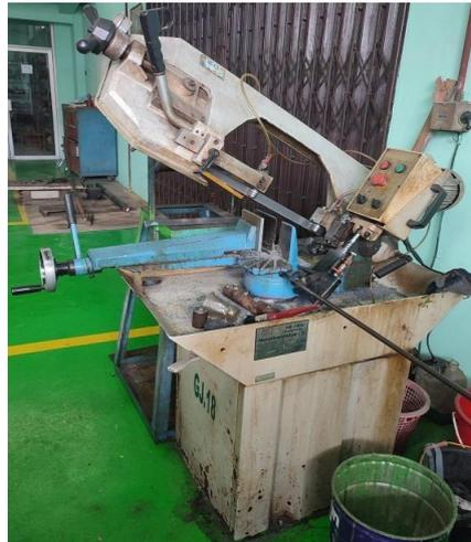
**Gambar 1.2. Mesin Gergaji *Horizontal Bandsaw***
