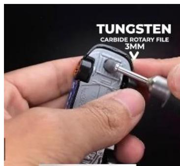
**Gambar 5. Membuka Rivet**
